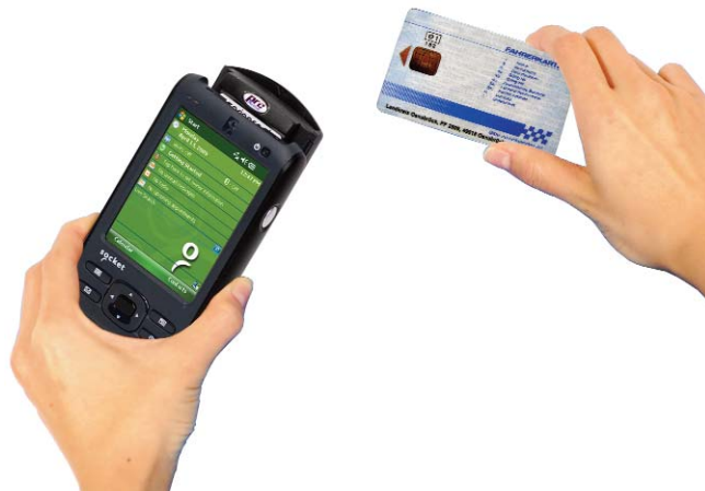
A Springcard smart card reader plugs into the SoMo to read the smartchip in a driver's card
